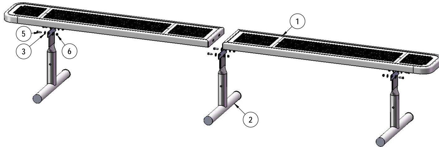
Attach the 10' Seat to the Legs as shown using specified hardware.
