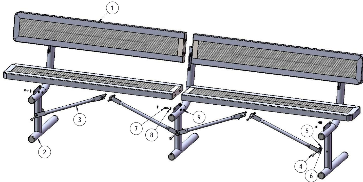
Attach the 29-1/2" Braces to the 940 legs as shown using specified hardware.
