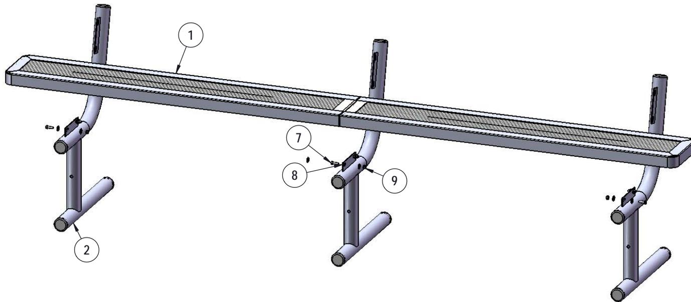
Attach the 10' Expanded Seat to the 940 legs using specified hardware.
