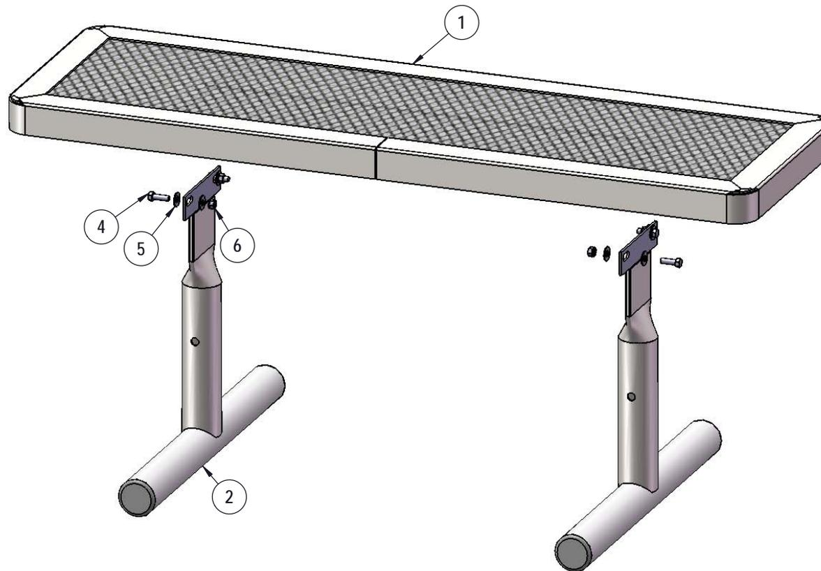
Attach the 4' Expanded Seat to the legs using specified hardware.
