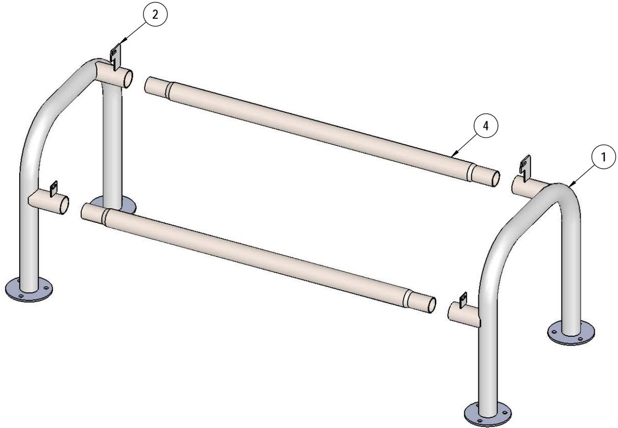
Slide the Spreader Tubes into the Legs.
