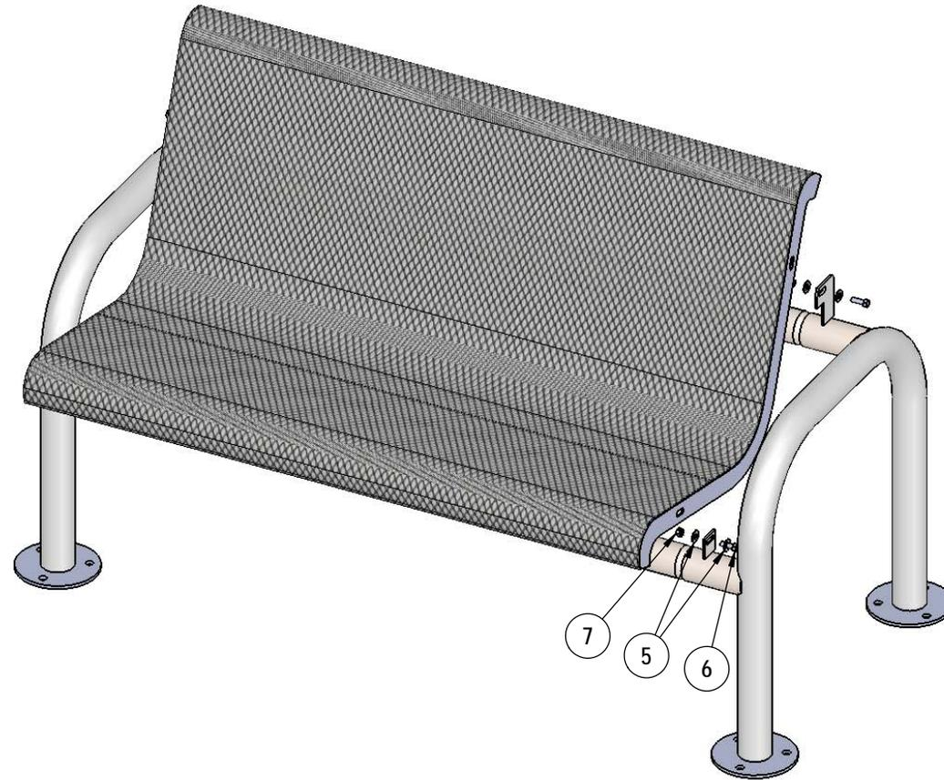
Attach the 4' Contour Seat to the Legs using specified hardware.
