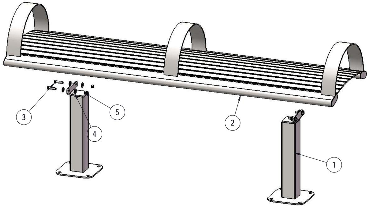
Recommended Surface Mount Hardware: 3/8" x 3-1/2" Concrete Expansion Anchor Bolts (Not Included)
