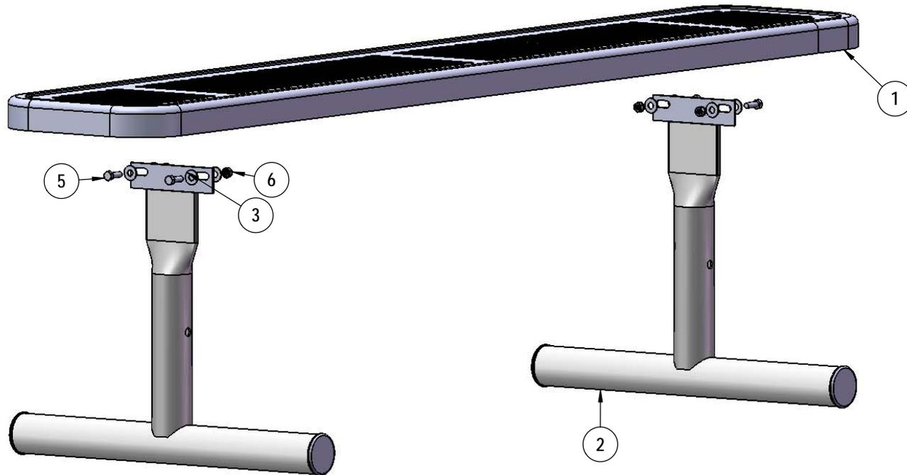
Attach the 6' Punched Seat to the Legs using specified hardware.
