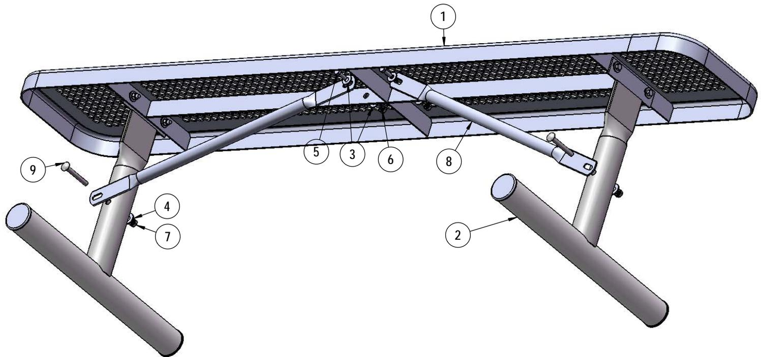
Attach the 26-3/4" Braces to the 6' Seat and Legs using specified hardware as shown.
