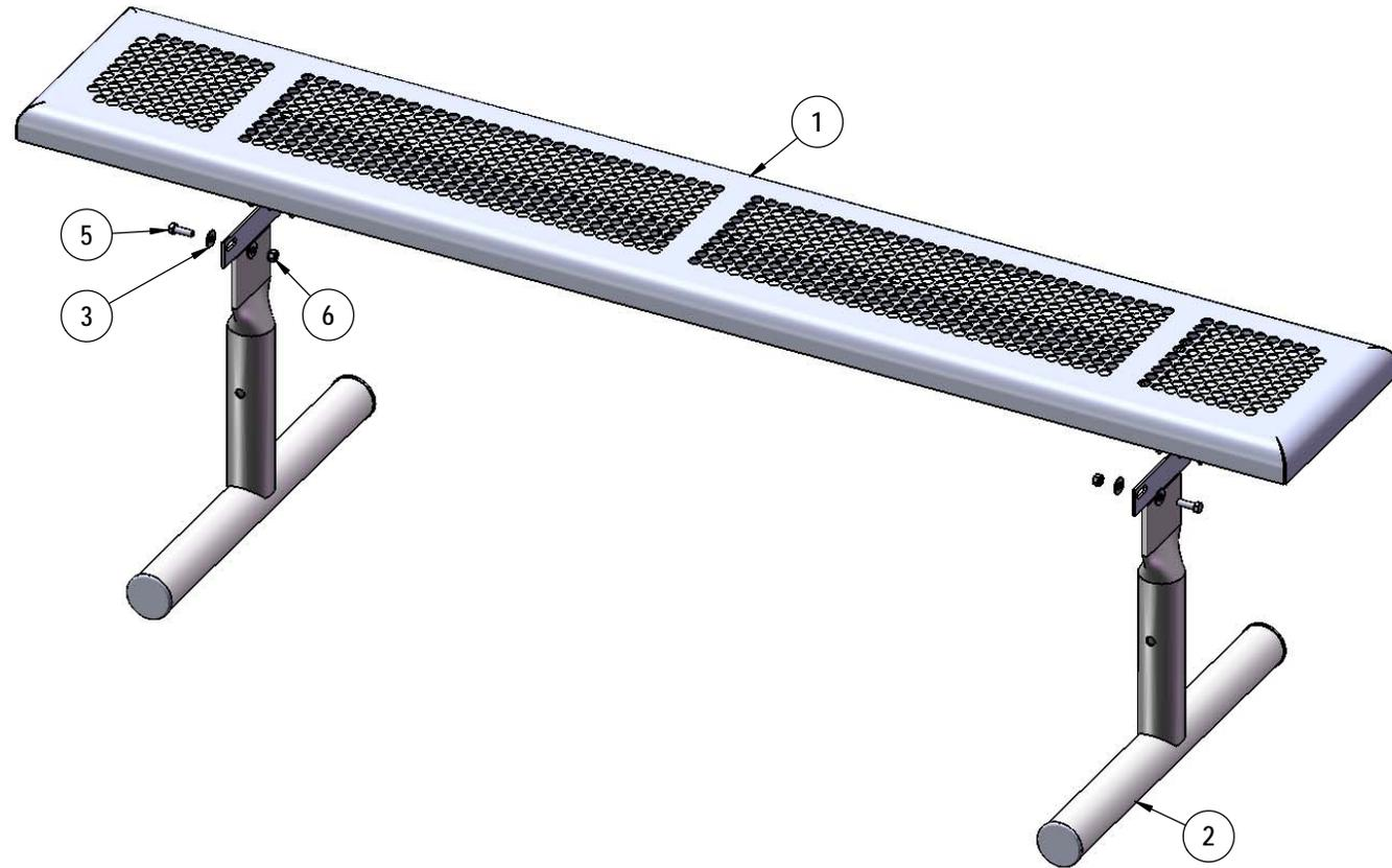
Attach the 6' Punched Rolled Seat to the Legs using specified hardware.
