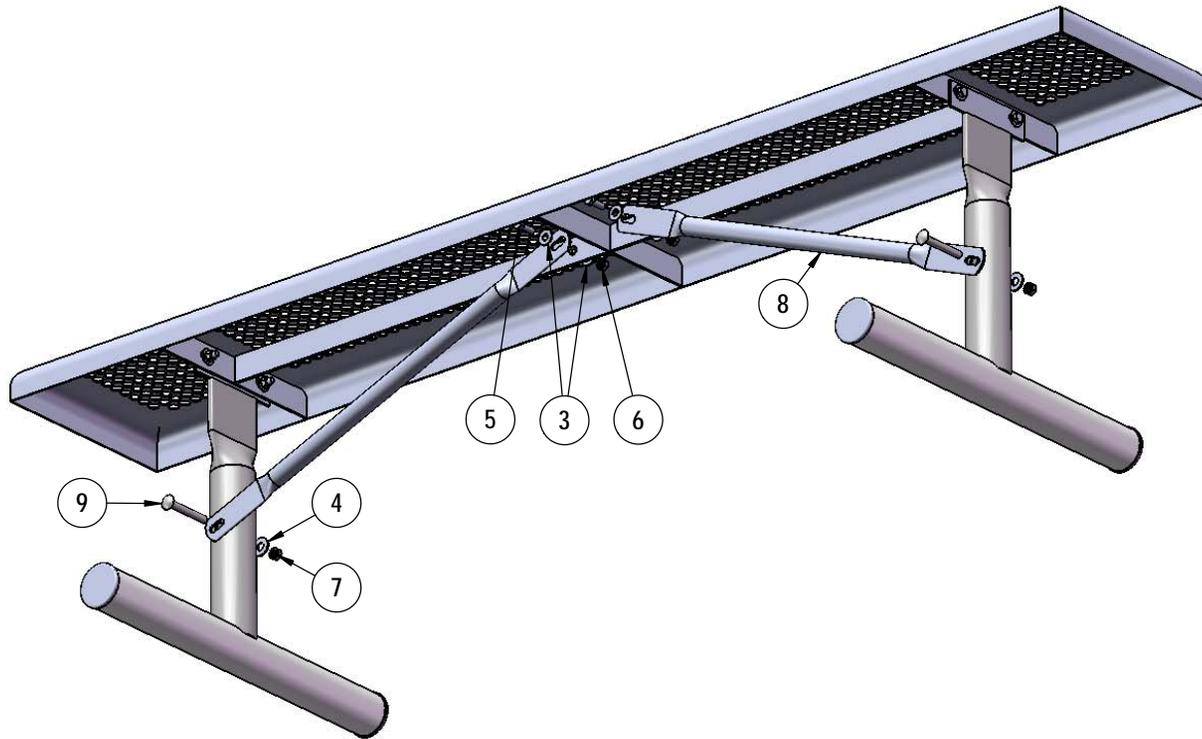
Attach the 26-3/4" Braces to the Legs using specified hardware as shown.
