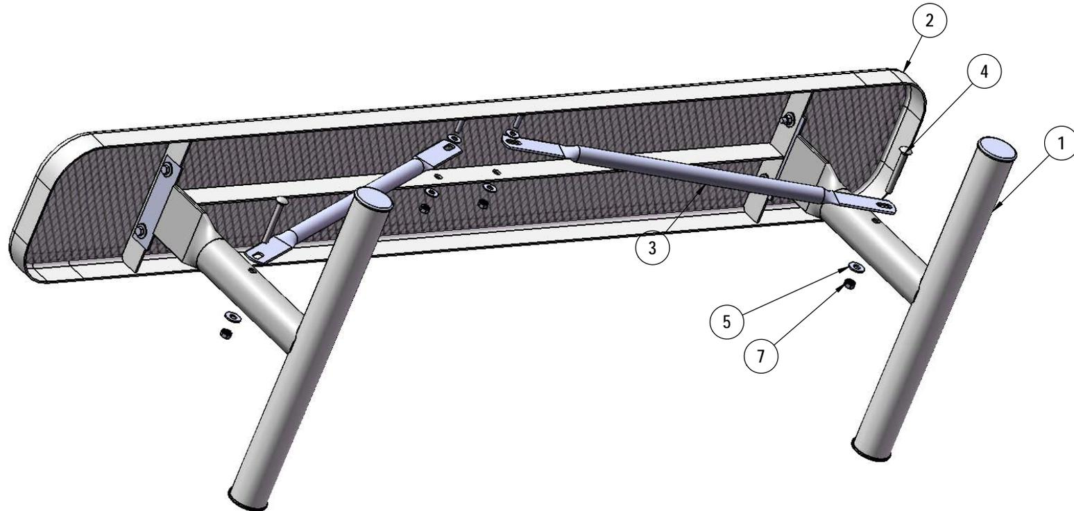
Attach 26 1/2" Brace to the legs as shown using specified hardware.
