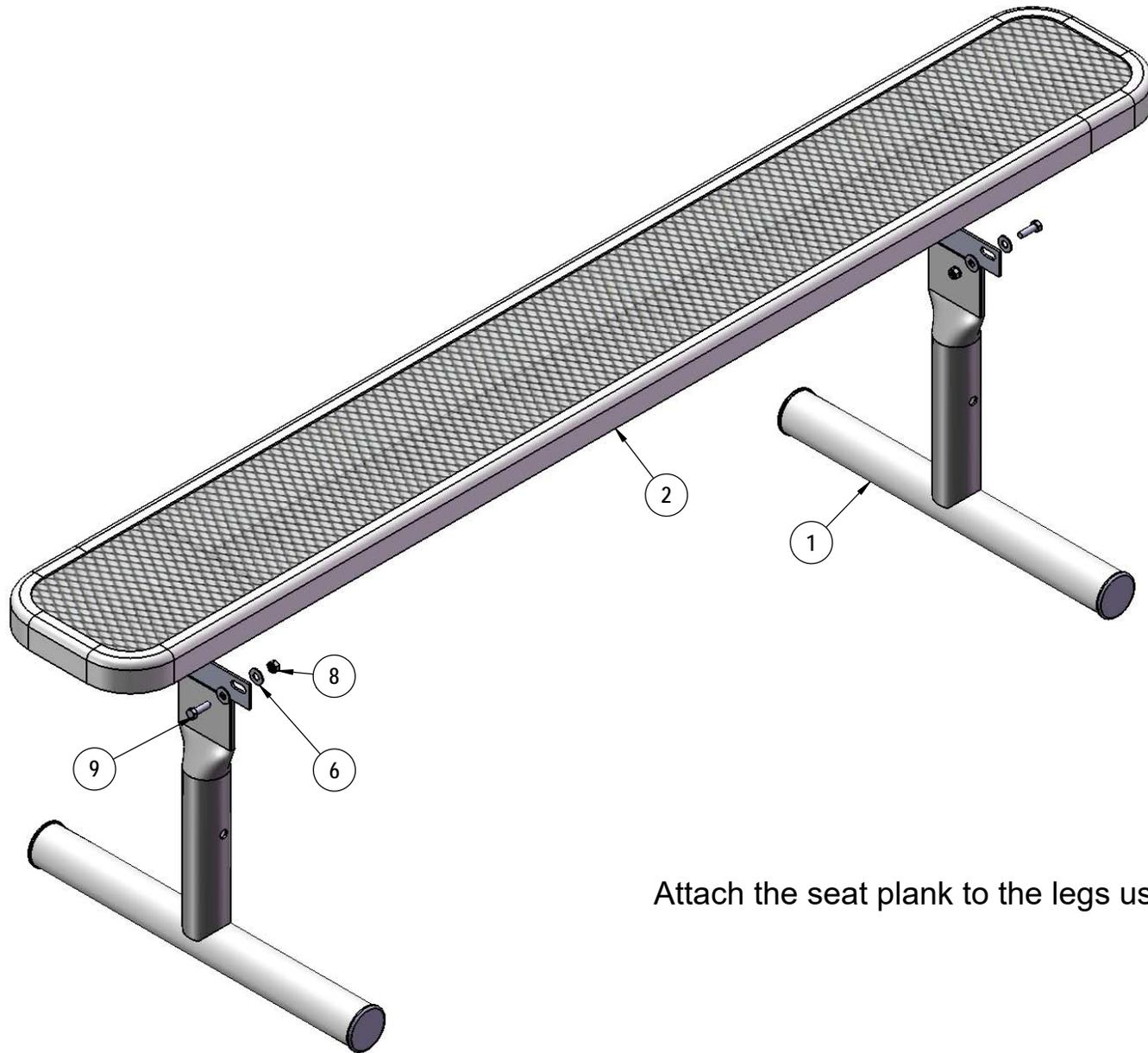
Attach the seat plank to the legs using specified hardware.
