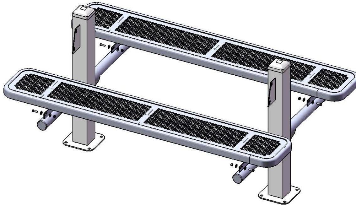
Attach the 6' Seats to the Legs using specified hardware.
