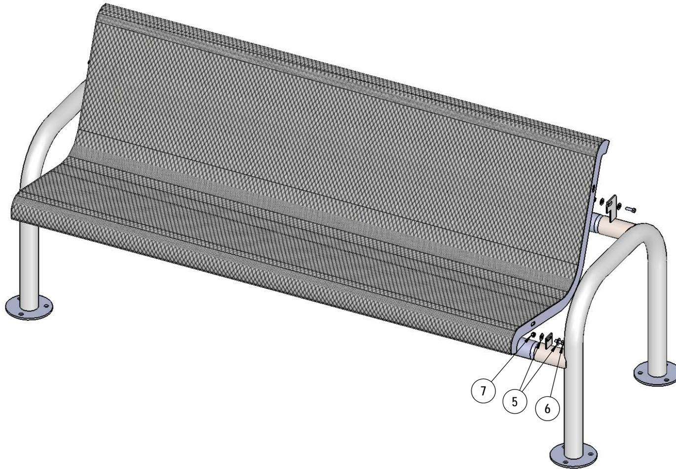
Attach the 6' Contour Seat to the Legs using specified hardware.
