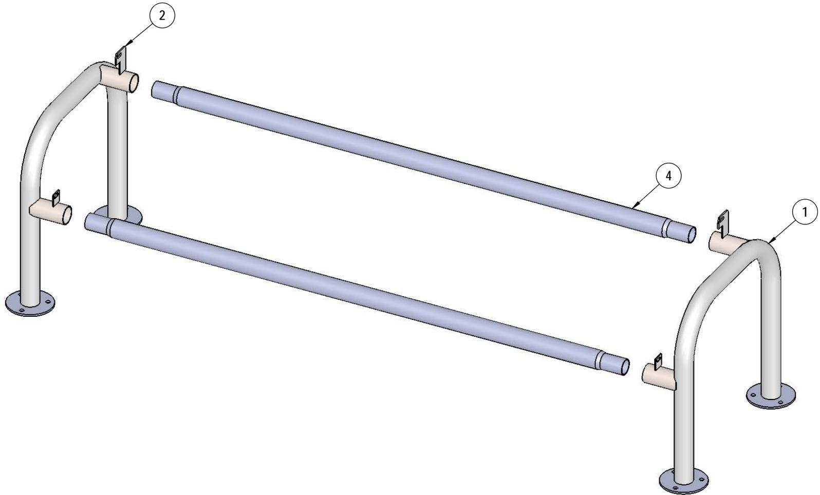
Slide the Spreader Tubes into the Legs.
