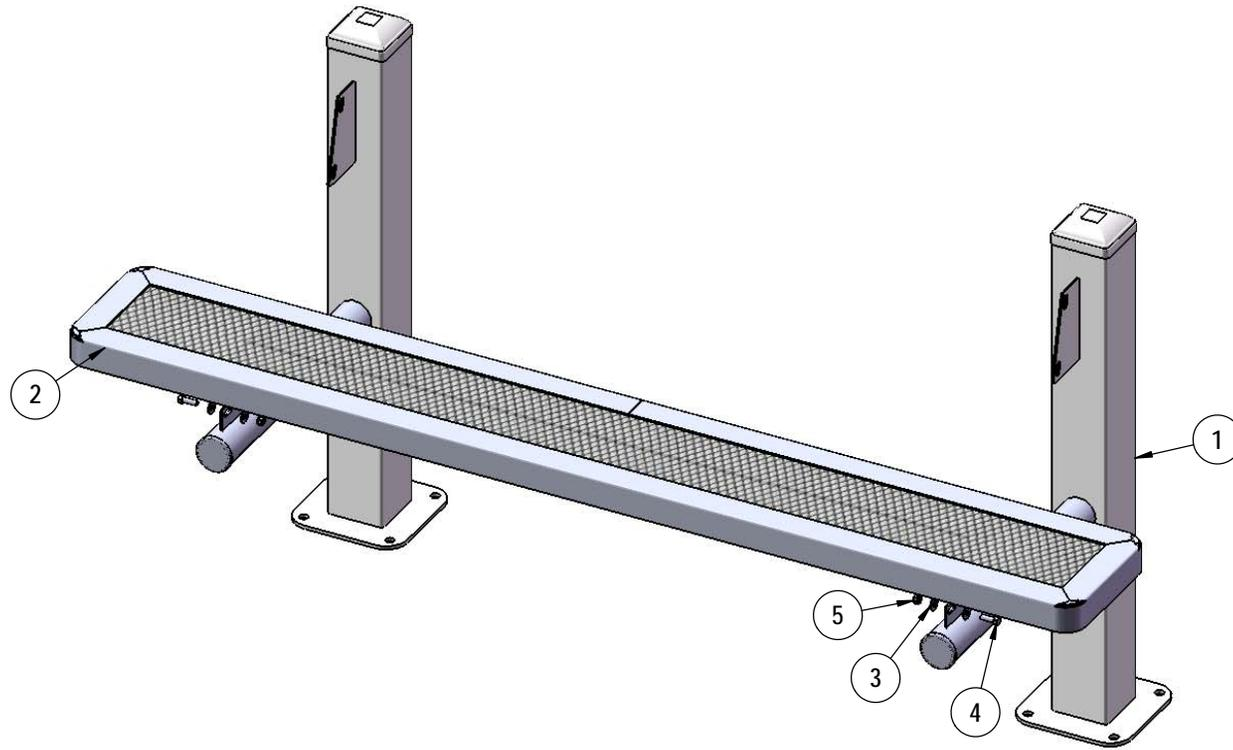
Attach the 6' Seat to the Legs using specified hardware.
