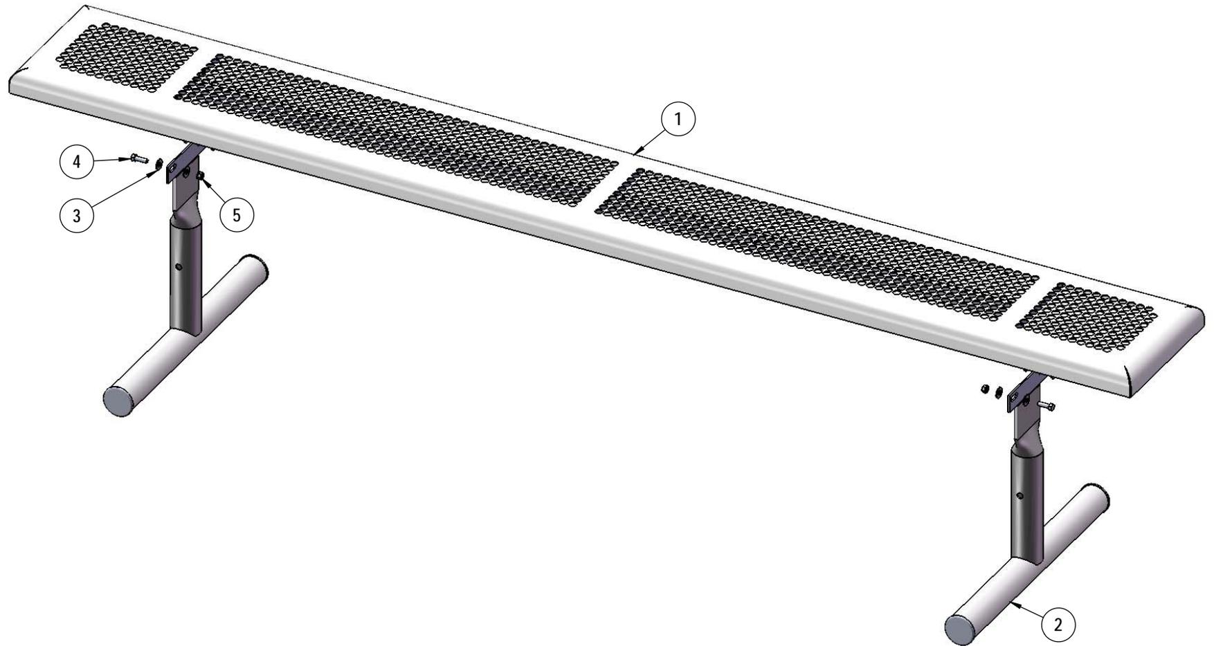
Attach the 8' Punched Rolled Seat to the Legs using specified hardware.
