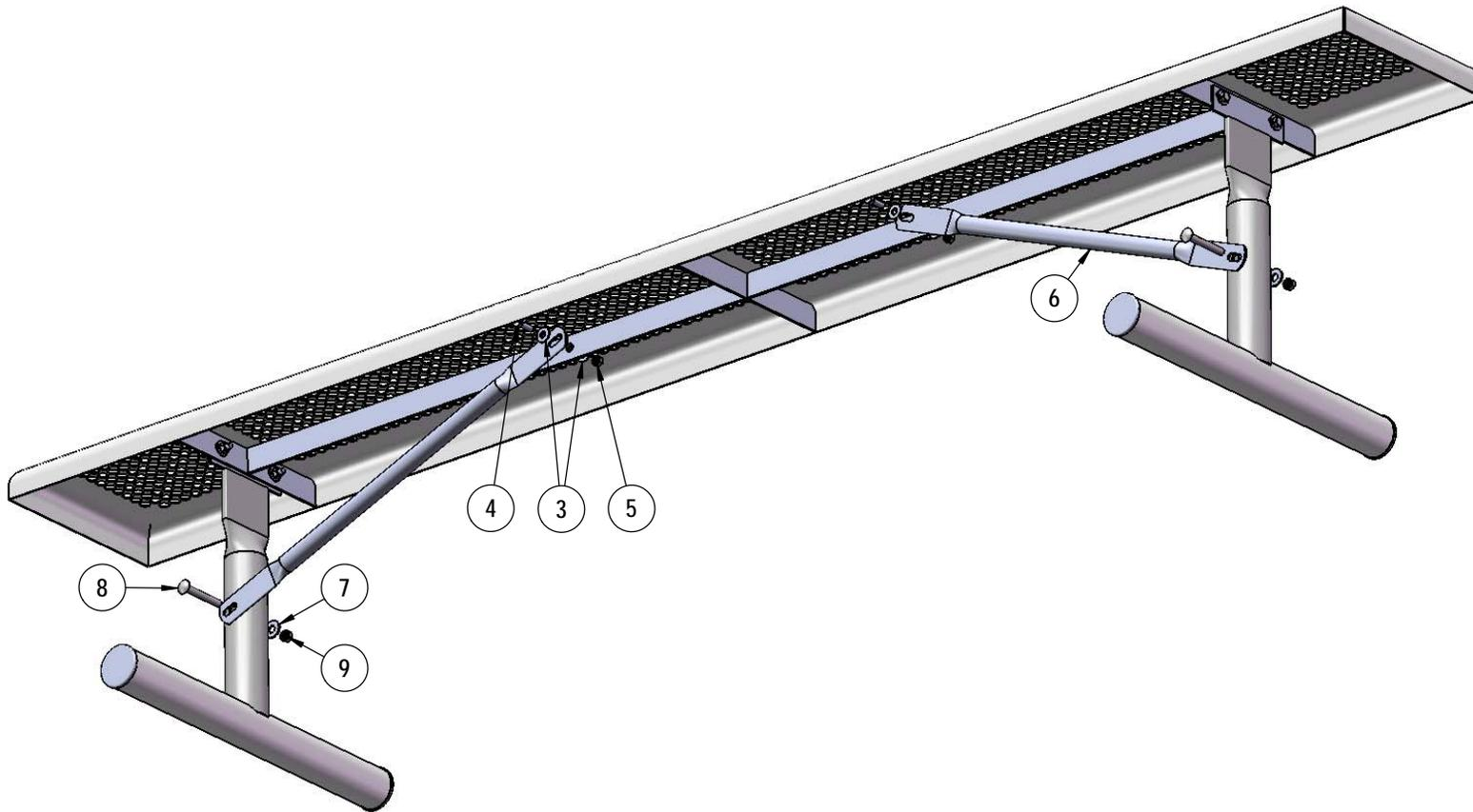
Attach the 26-3/4" Braces to the Legs using specified hardware as shown.
