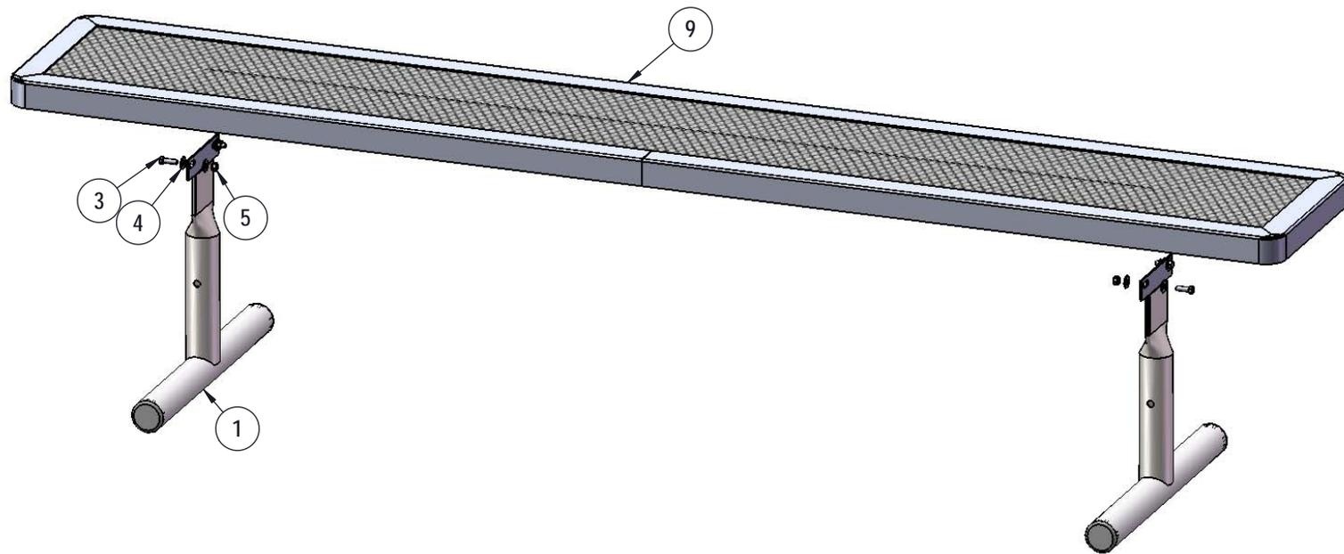
Attach the 8' Expanded Seat to the legs using specified hardware.
