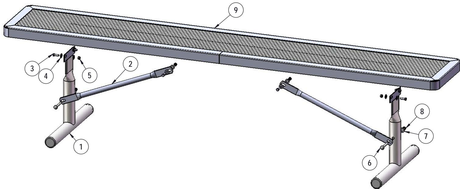
Attach the 29-1/2" Braces to the legs as shown using specified hardware.
