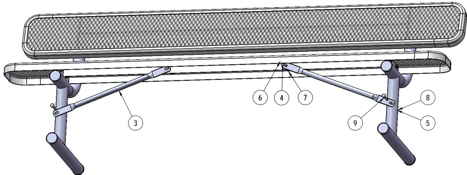
Attach the 26 3/4" Braces to the legs as shown using specified hardware.
