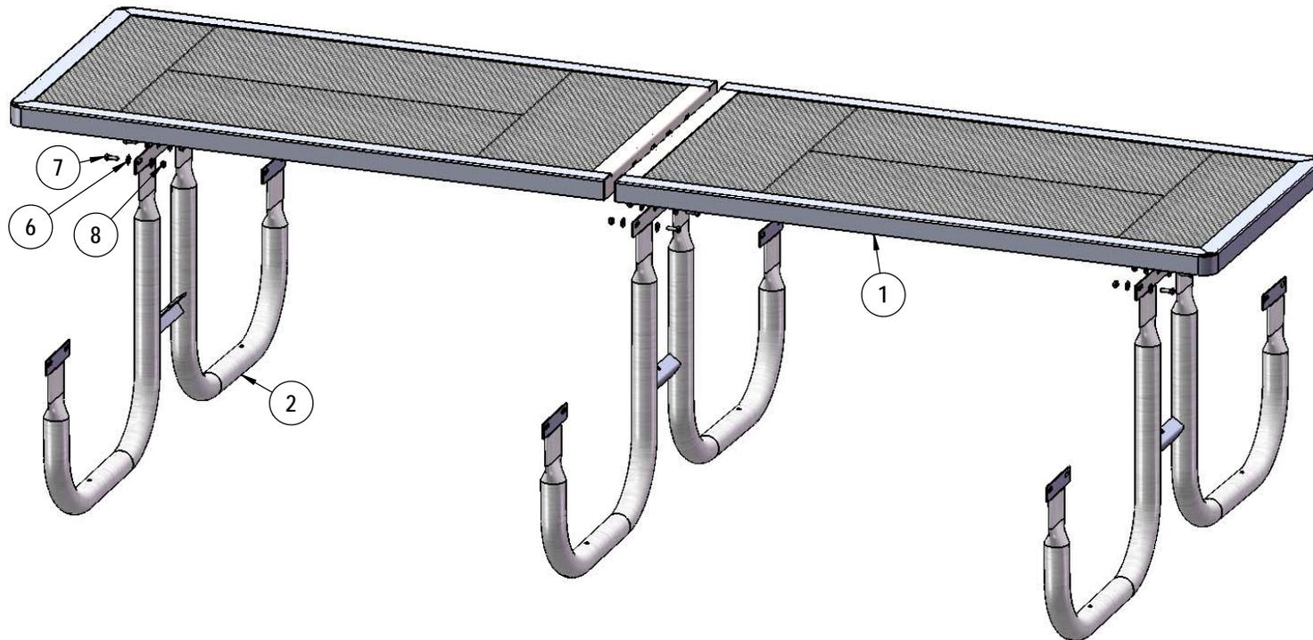
Attach the top to the top legs as shown using specified hardware.
