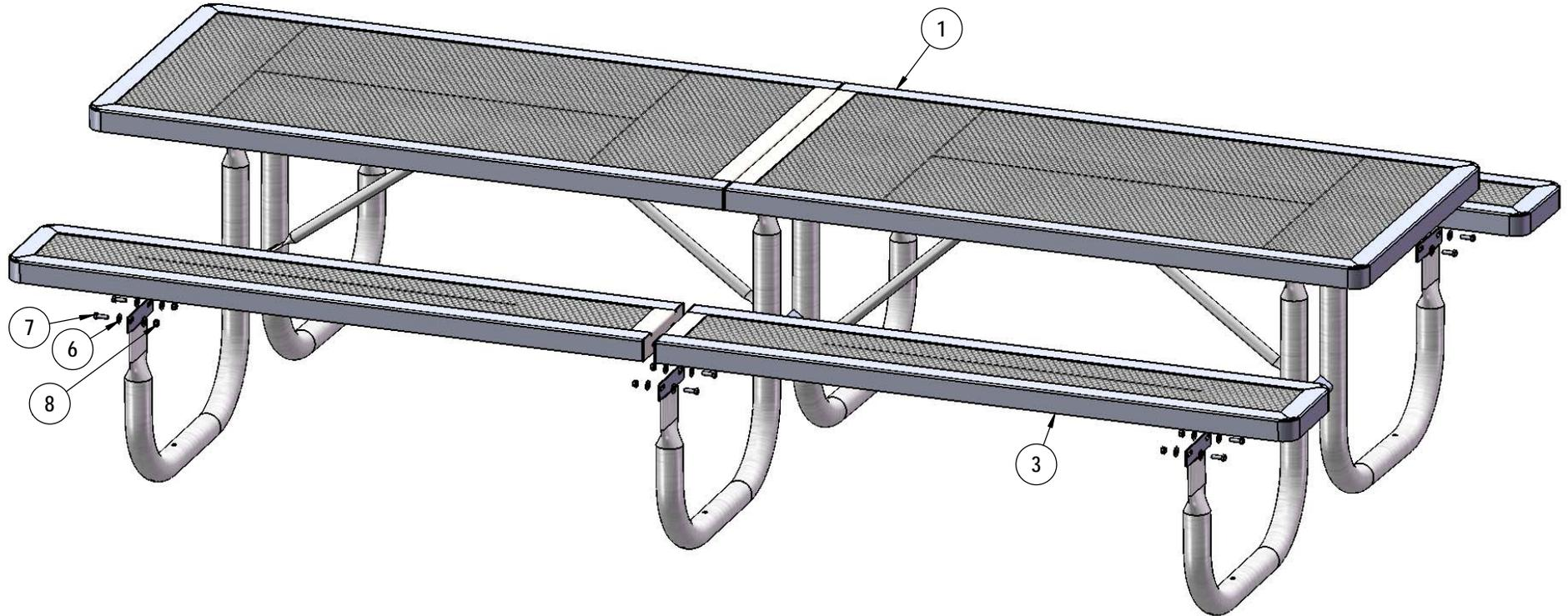
Attach the seats to the frame as shown using specified hardware.
