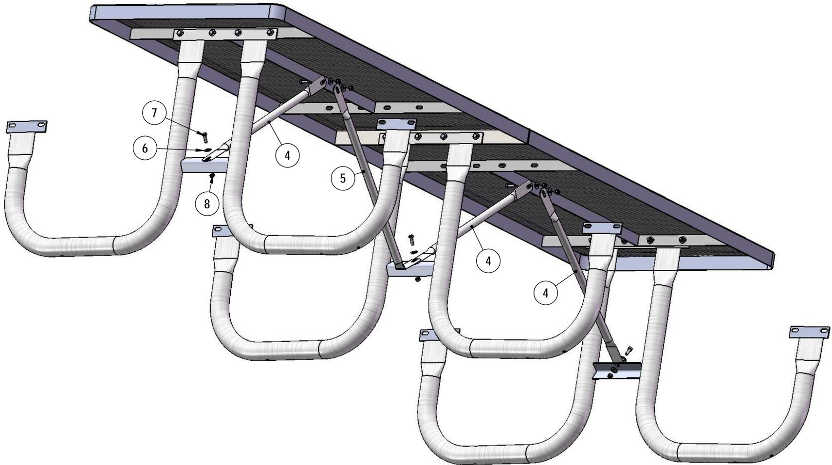
Attach the braces to the frame and under side of the top as shown using specified hardware.
