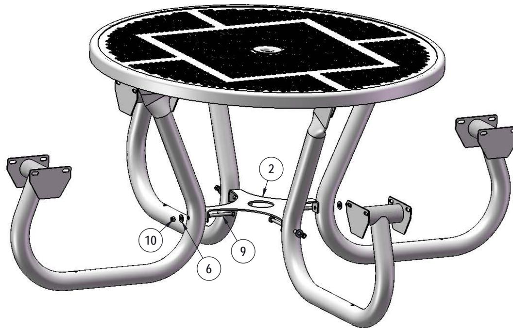
Attach the Spreader Plate to the Legs as shown using specified hardware.
