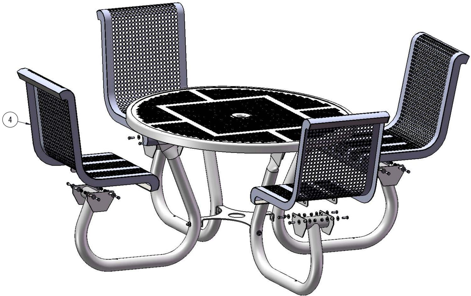
Attach the Seats to the Frames as shown using specified hardware.
