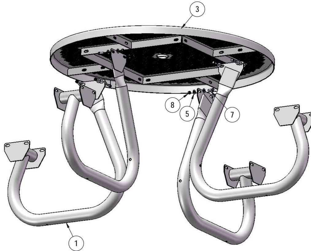
Attach the Top to the Legs as shown using specified hardware.
