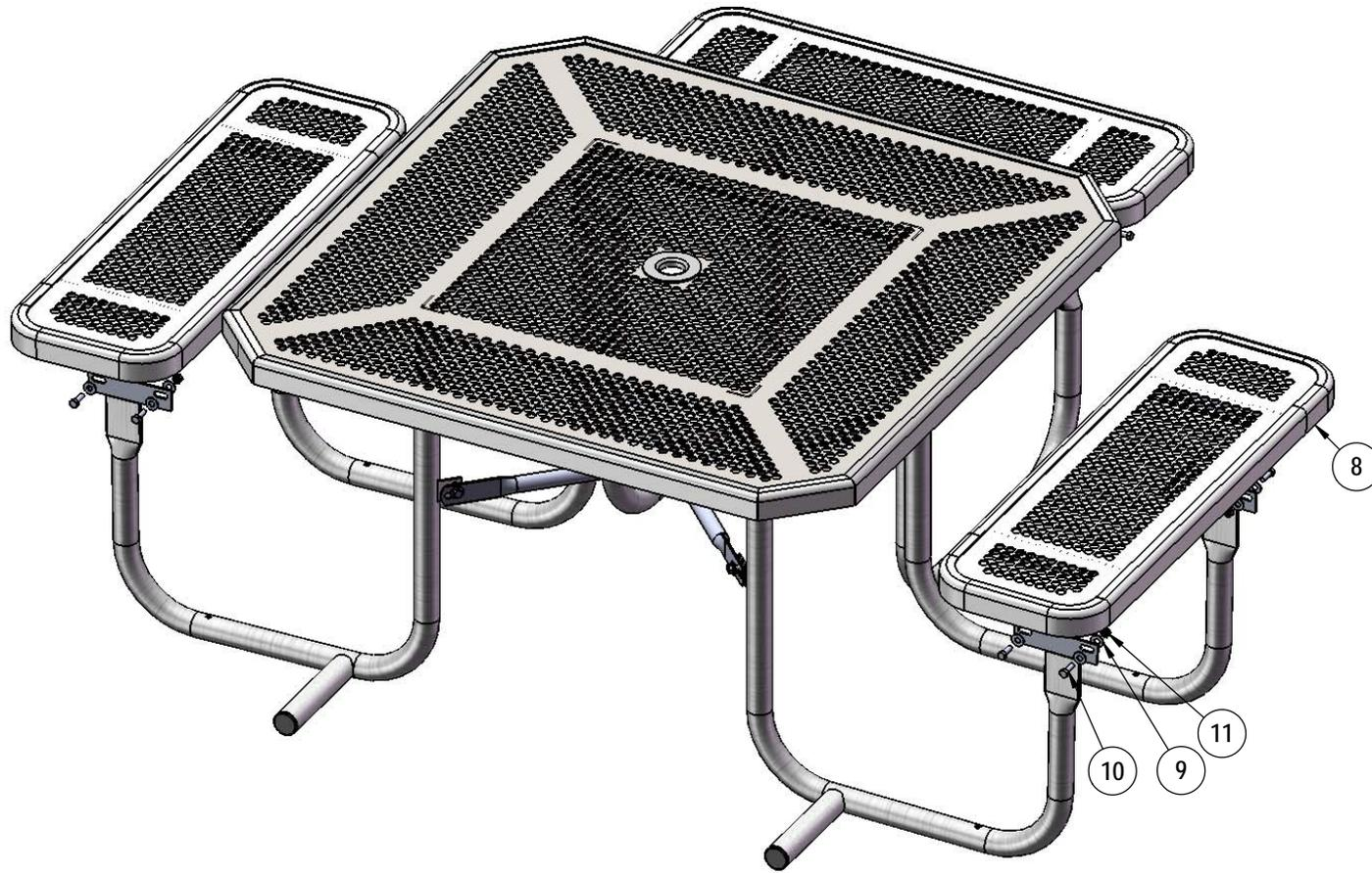
Attach the 3' Seats to the Legs using specified hardware.
