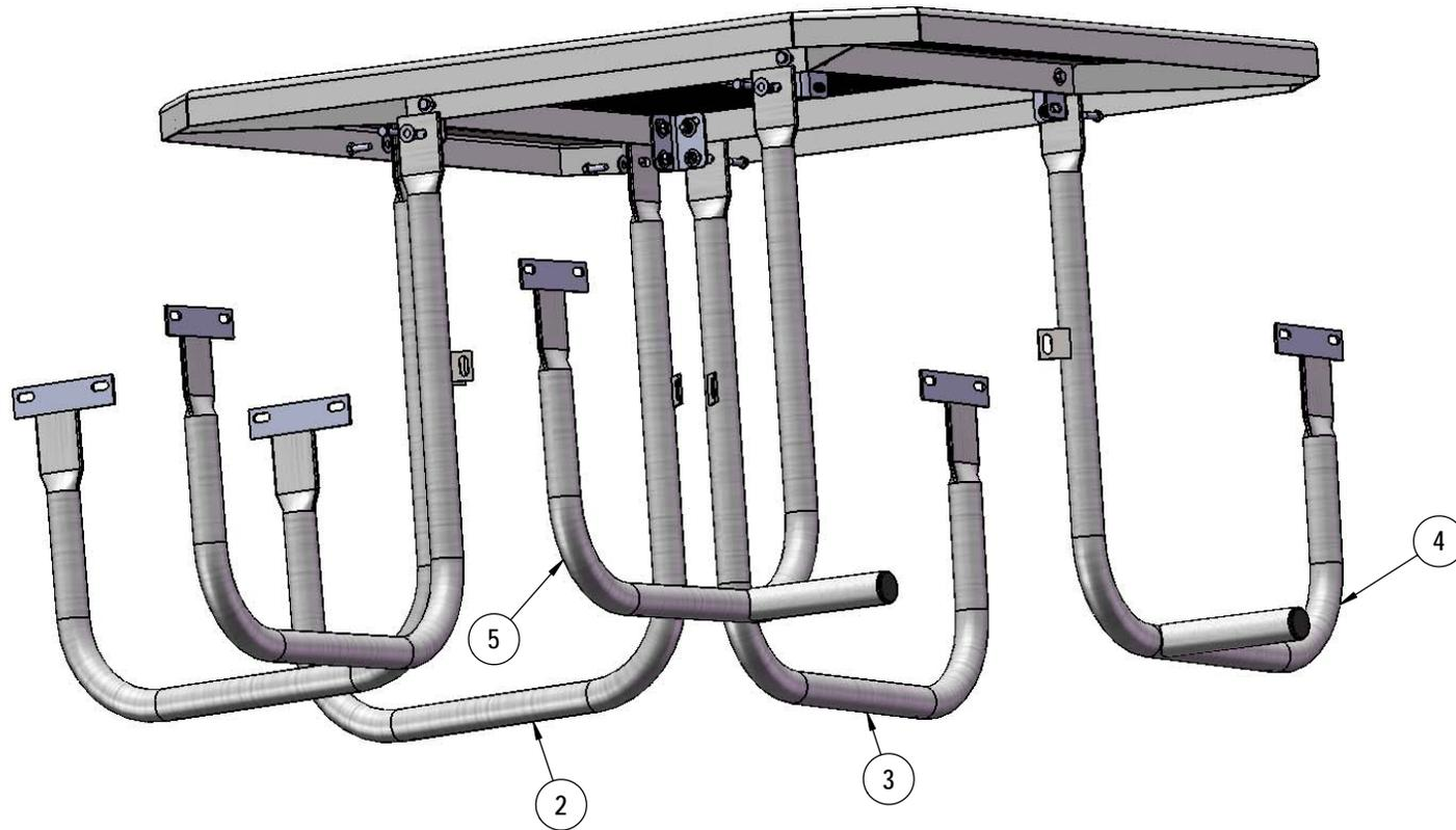
Attach the Legs to the Extension Tabs using specified hardware.
