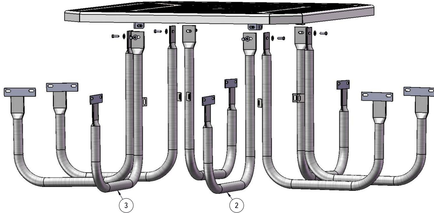
Attach the Legs to the Extension Tabs using specified hardware.
