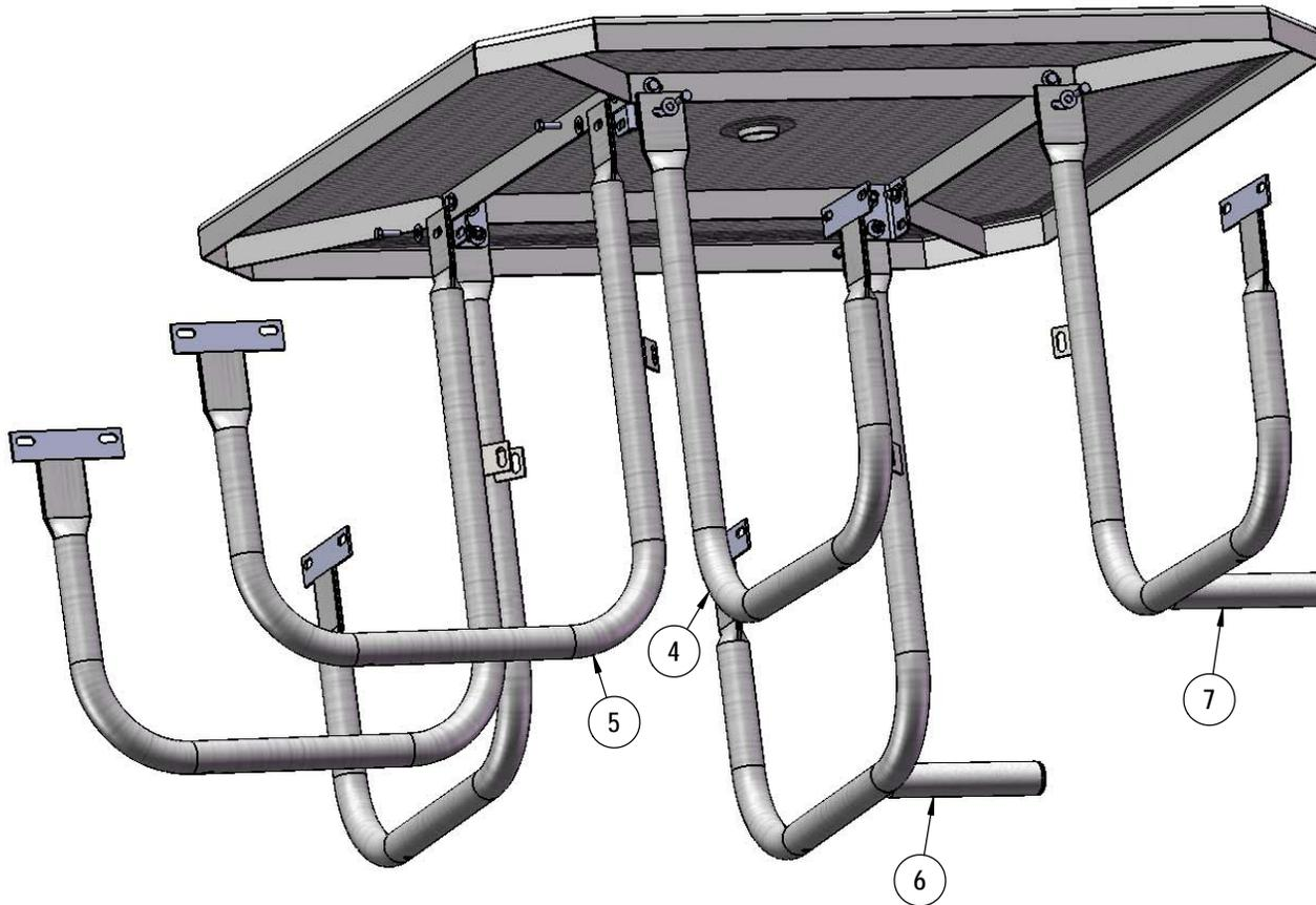
Attach the Legs to the Extension Tabs using specified hardware.
