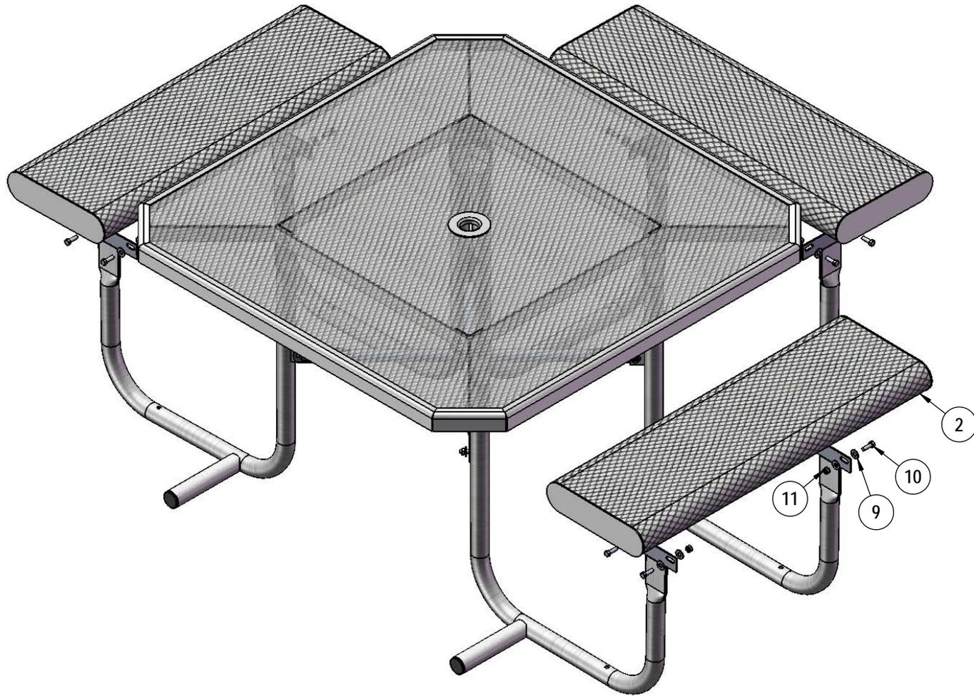
Attach the 3' Seats to the Legs using specified hardware.
