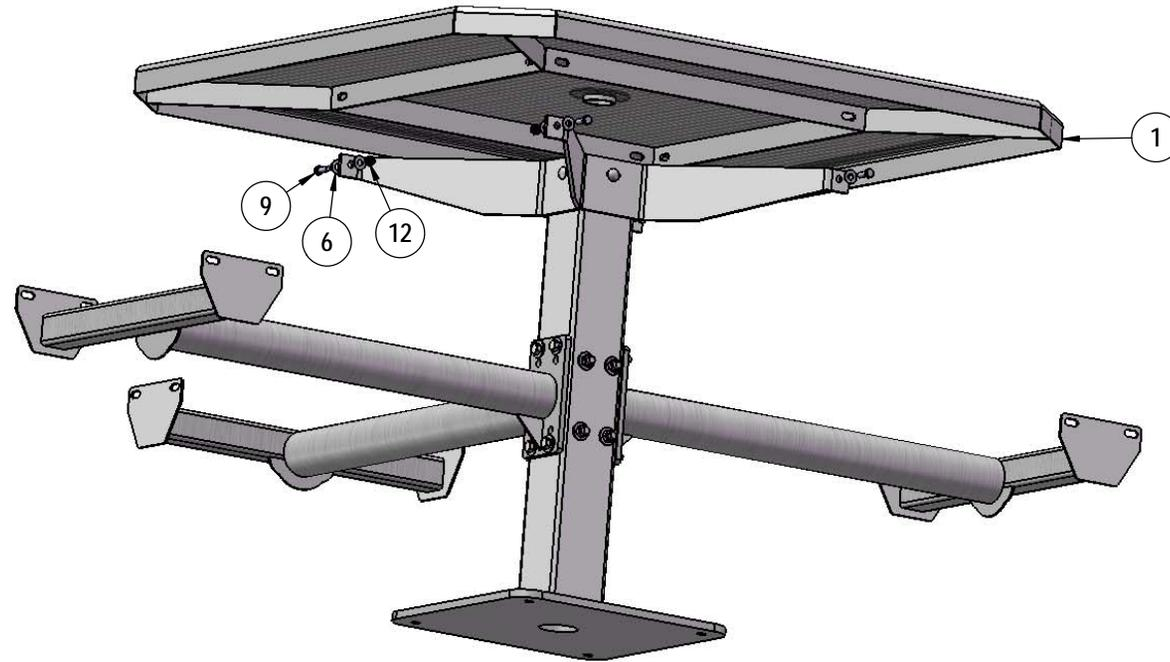
Attach the 46" Octagon Top to the H Bracket using specified hardware.
