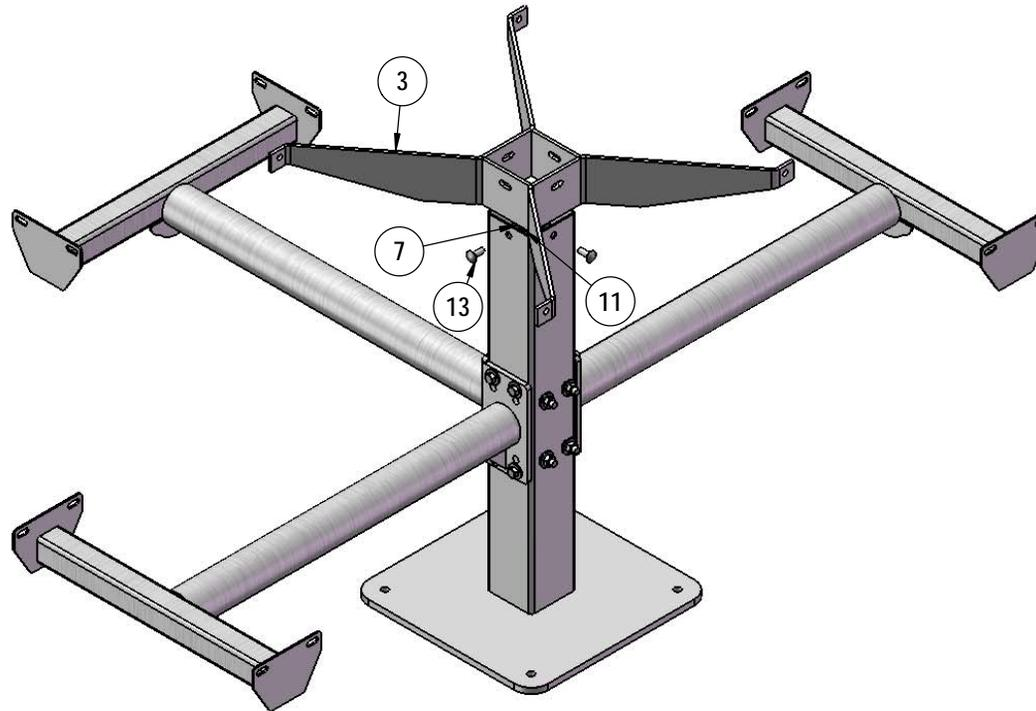
Attach the H Bracket to the Post using specified hardware.
