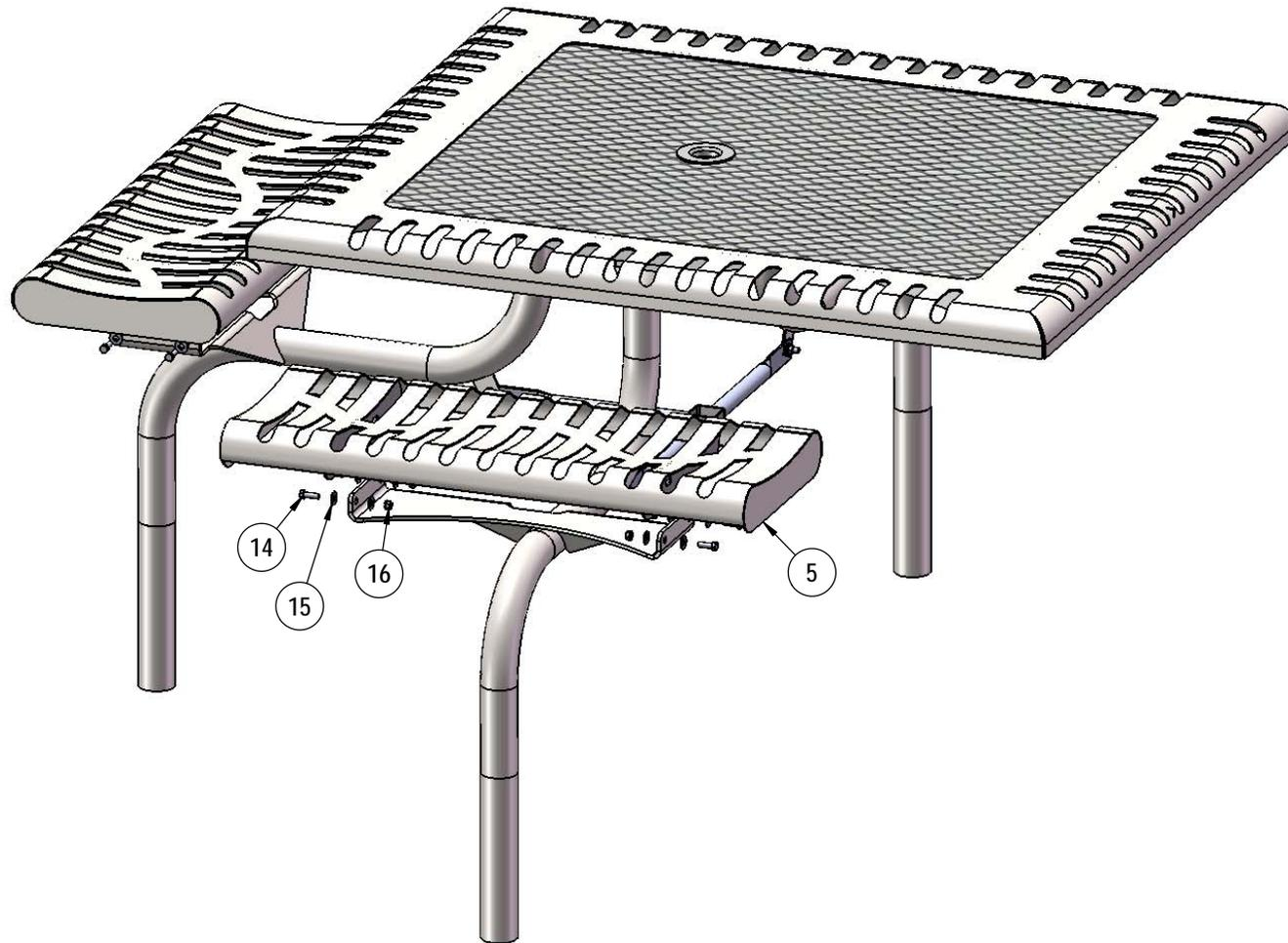
Attach the seats to the legs as shown using specified hardware.
