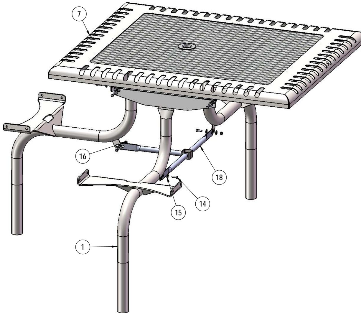
Attach the legs to the top as shown using specified hardware. Then attach the cross brace to the legs.
