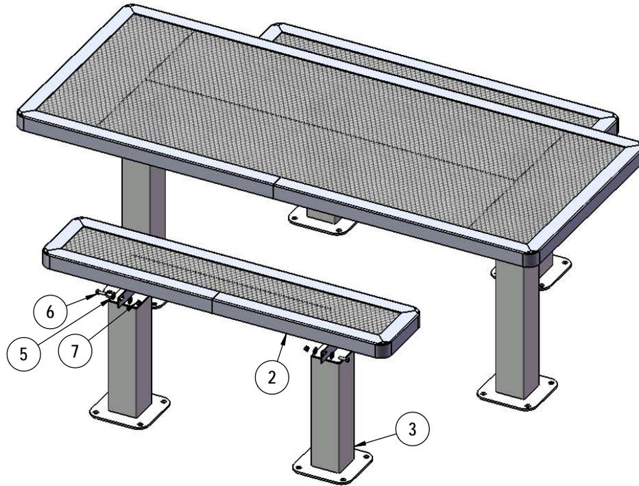
Attach the seats to the seat legs as shown using specified hardware.
