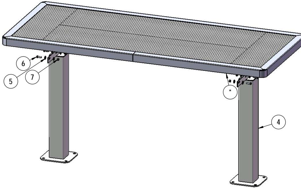
Attach the top to the top legs as shown using specified hardware.
