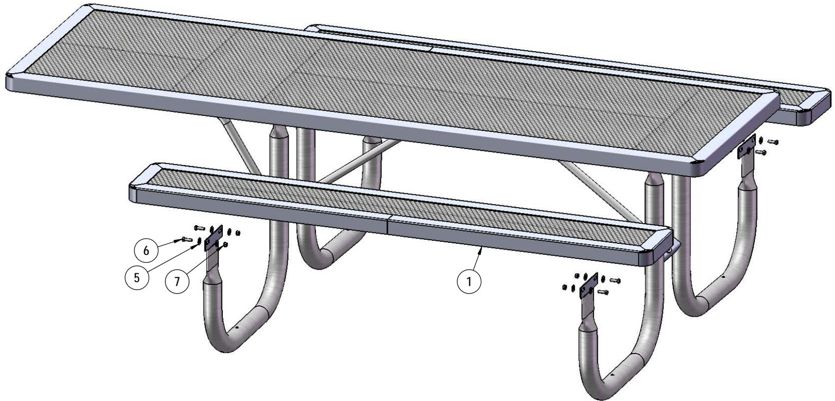
Attach the seats to the frame as shown using specified hardware.
