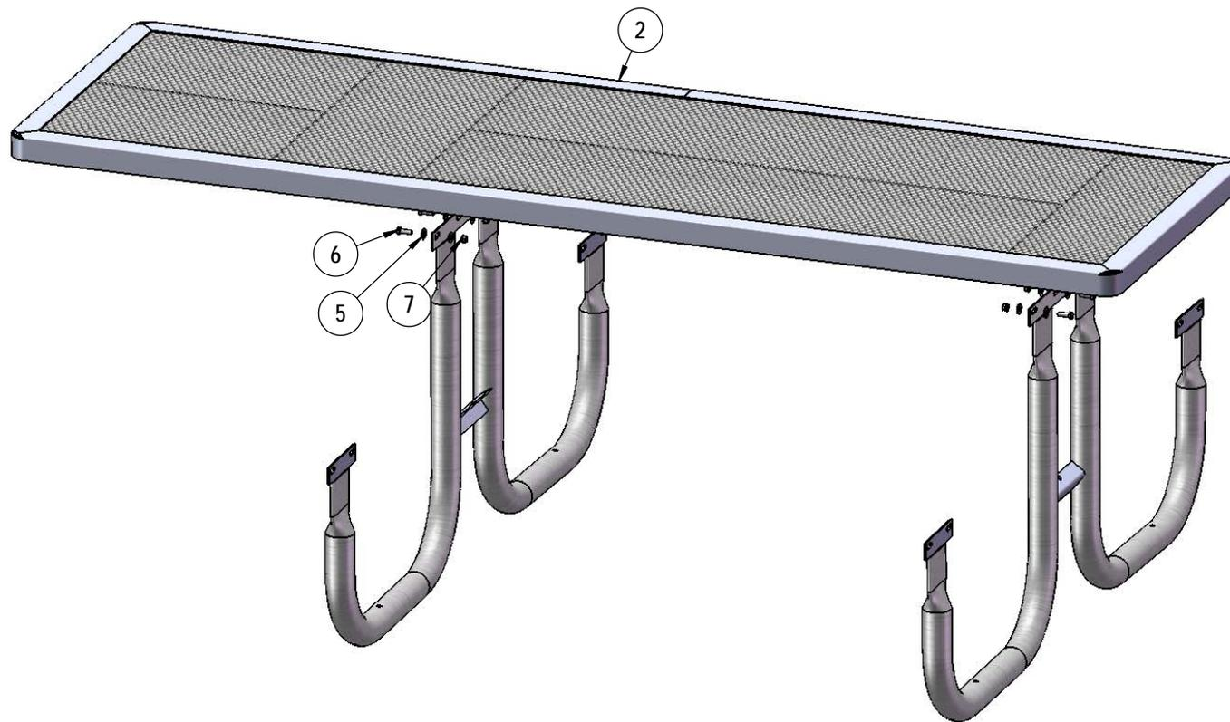
Attach the top to the top legs as shown using specified hardware.
